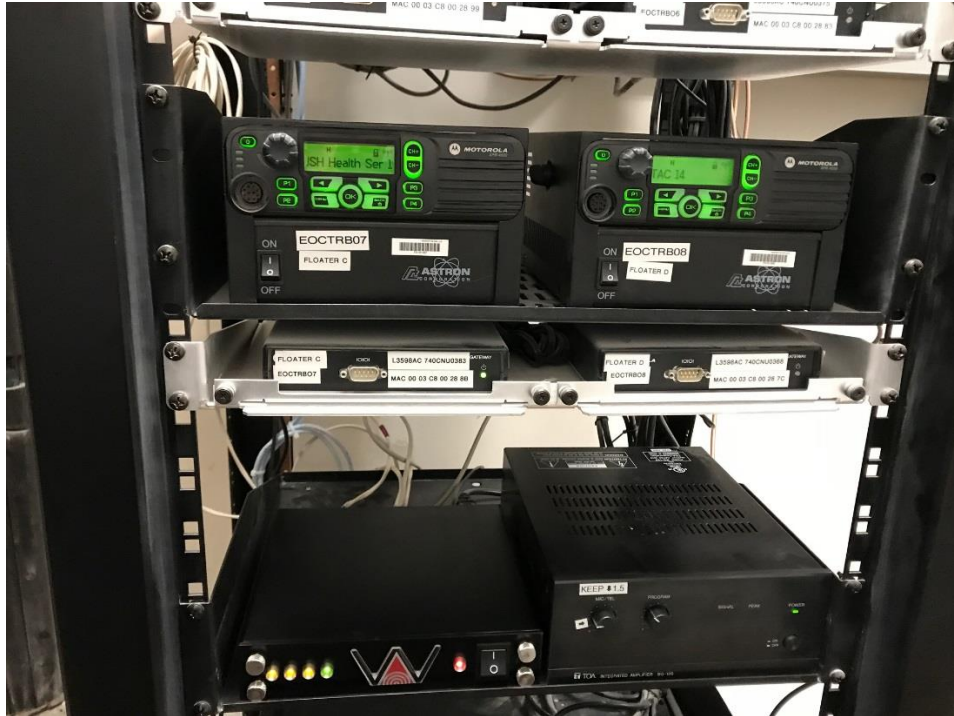
This picture depicts the early warning lab device connected to the station announcement system and garage door opener
