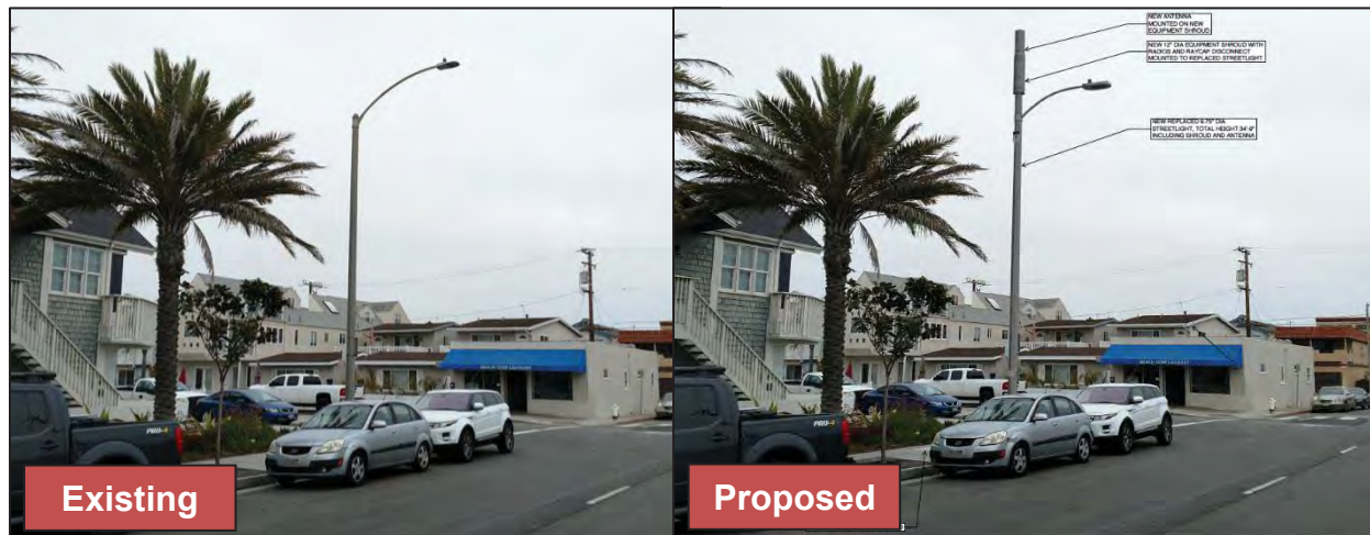
Figure 1, Existing photograph (left) with proposed rendering (right) showing the replaced streetlight pole, antenna, equipment shroud, and below-grade equipment handholes.
