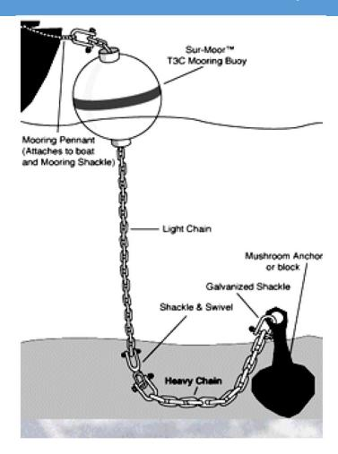
The diagram shows the typical configuration of an offshore mooring in Newport Harbor. A single two-point mooring will typically use two of the mooring configurations shown. One for the bow of the boat and one for the stern.
