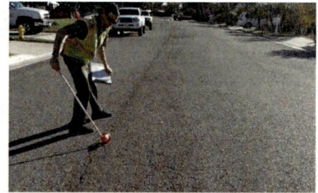
Figure 8: GMU Staff Engineer performing a PCI survey.
