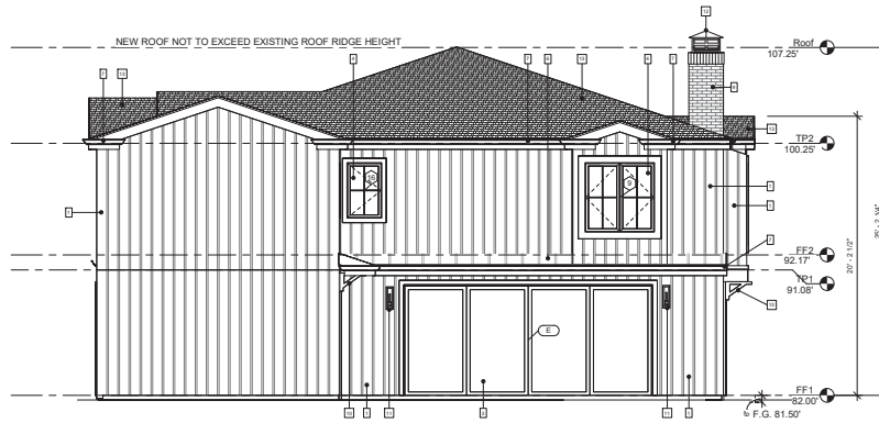
2 REAR EXTERIOR ELEVATION 1/4" = 1'-0"
