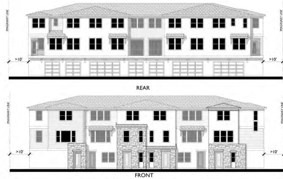
ALL BUILDING TYPE 'A' 3-STORY CONDOMINIUMS ON SITE EQUIP WITH SPRINKLERS AND EXCEED MINIMUM FIRE SEPARATION DISTANCE OF 10 FEET AND ALLOWABLE FOR UNLIMITED OPENING PER C.B.C. SECTION 705.9.1 EXCEPTION 2
