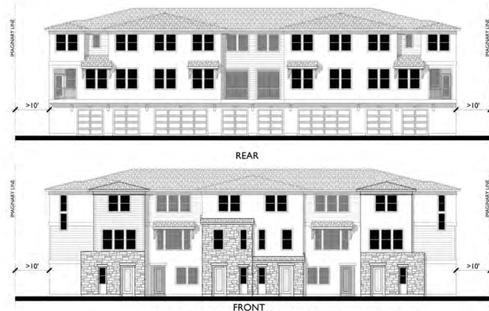
ALL BUILDING TYPE 'B' 3-STORY CONDOMINIUMS ON SITE EQUIP WITH SPRINKLERS AND EXCEED MINIMUM FIRE SEPARATION DISTANCE OF 10 FEET AND ALLOWABLE FOR UNLIMITED OPENING PER C.B.C. SECTION 705.9.1 EXCEPTION 2
